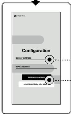
Set the target address at the format below: `http(s)://192.168.10.250/display`.
