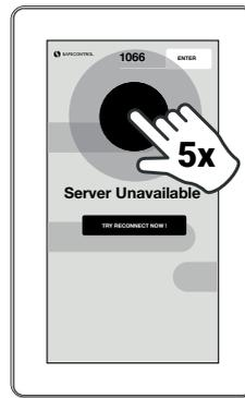
To enter the service menu, tap the display 5-times in quick succession. The window for entering the PIN code will appear "1066".
