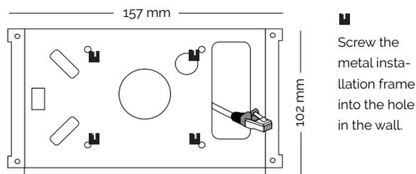
■ Screw the metal installation frame into the hole in the wall.
